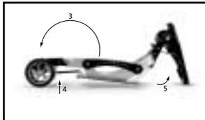
**STEP 3 - 4** - Continue to open the **front wheel assembly**, making sure the **cable connector pin** stays on top of **main deck**. Lock **cable connector pin** into slot on **main deck**.
