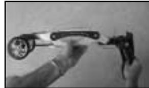
**STEP 2** - Fold the **tail/rear assembly** clockwise.
