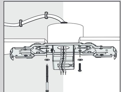
**Use wood screws** (included) when securing to support structure with approved electrical outlet box. Drill 9/64" pilot holes in support structure to aid in securing ceiling bracket with hardware found in the ★ hardware bag.
