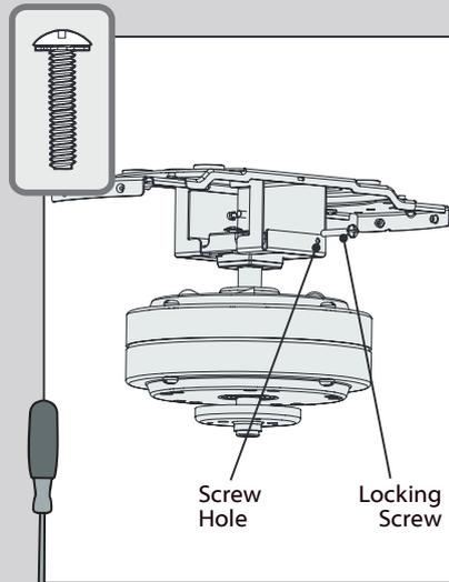
⊗ Once the motor is in the ceiling bracket, use the two locking screws found in the ★ hardware bag to secure the motor to the ceiling bracket.
