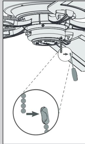
Connect the fan pull chain pendant to the short chain coming from the switch housing.
