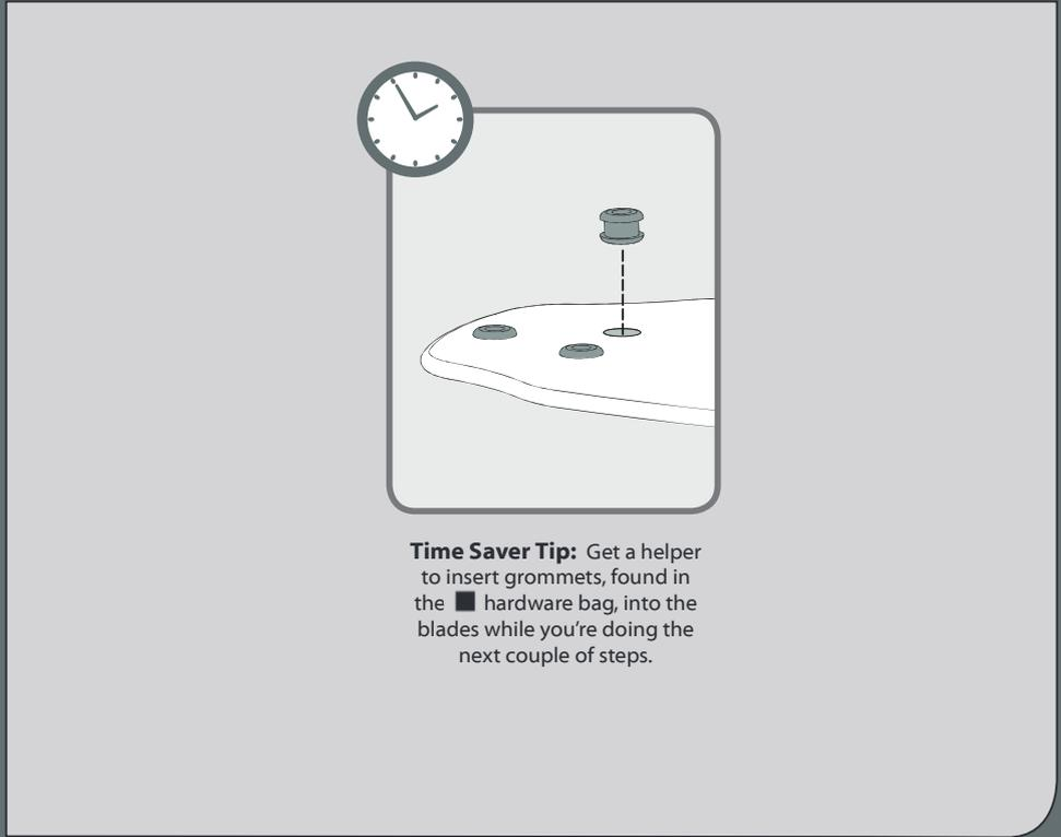
**Time Saver Tip:** Get a helper to insert grommets, found in the ■ hardware bag, into the blades while you're doing the next couple of steps.
