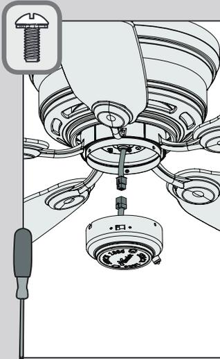
⊗ Partially install two of the switch housing screws found in the bag. Connect the plugs from the upper and lower switch housings. Make sure to line up the colored markings on the plug connectors.
