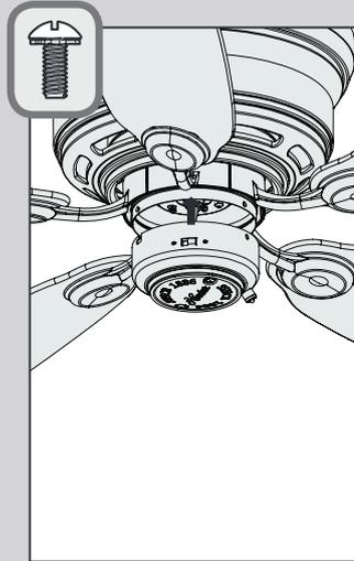
Align the notches in the sides of the lower switch housing with the screws on the upper switch housing. Twist the lower switch housing clockwise to lock into place. Install the third switch housing screw. Tighten all three screws securely.
