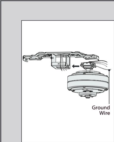
While holding the wires out of the way, lift the motor assembly and place the square hanger into the opening in the ceiling bracket. Be sure the ground wire attached to the hanger faces out of the large opening in the ceiling bracket.
