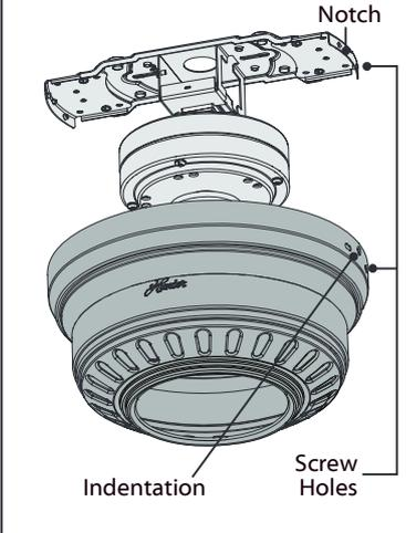
Raise the motor housing up over the motor and ceiling bracket. Turn the motor housing so the screw holes align and the indentation in the housing locks into place with the notch in the ceiling bracket. **The motor housing is not secured until the next step is complete. Do not leave unattended.**
